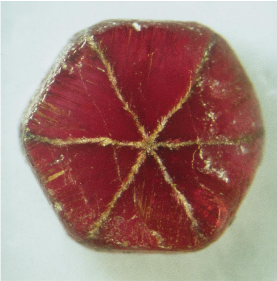
Fig. 2. An example of trapiche ruby showing textures, with polished (0 0 0 1) surface. Sample B, about 3.3 mm across.
