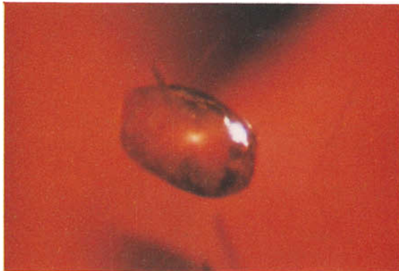
FIG. 3. Round zircon crystal with high relief, inside a sapphire from Umba Valley. 80x . (light-field illumination).
