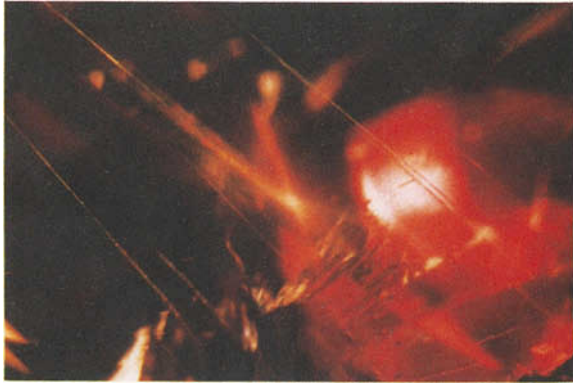
FIG. 1. Survey of the most typical internal scene, pressure parting lines in Umba Valley sapphire of reddish-brown colour. 40x . (dark field illumination).
