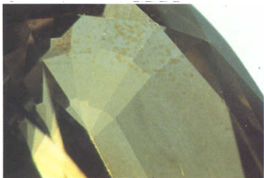
Fig. 2. Using diffused transmitted light on this same sapphire reveals an orangy-yellow coloured halo surrounding each of the minute whitish-appearing acicular inclusions. 25x.
