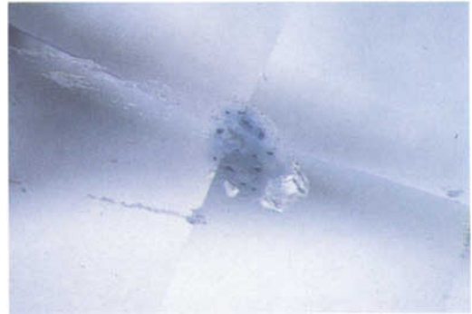
Fig. 5. (Above right) This tight grouping of irregular titaniferous hematite crystallites has released both titanium and iron during heat treatment resulting in the surrounding zone of blue colour in this Sri Lankan Sapphire. Diffused transmitted light. 40x.
