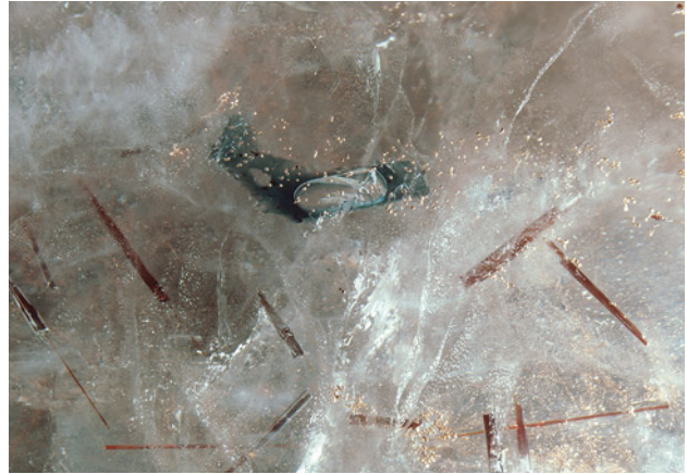
Figure 13. A suite of columbite rods, copper crystals, and a large air bubble seen within a film of blue flux liquid. Photomicrograph by Jamie Price; field of view 7.19 mm.
