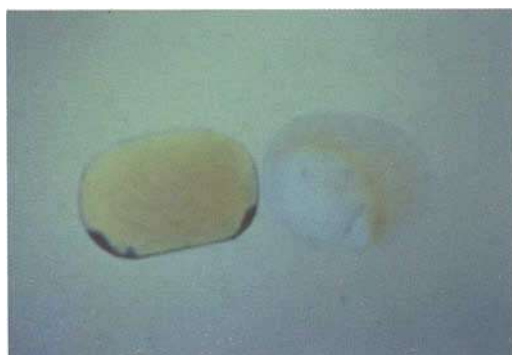
Fig. 2. The same two stones from Fig. 1, but now with a blue filter placed below the immersion cell. The blue filter provides contrast between the colour zoning and the background, making it much easier to resolve.
