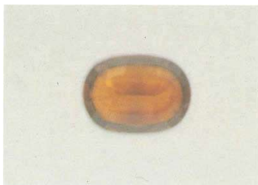
Fig. 4. The same stone from Fig. 3 is now shown just after it was exposed within 1 cm to the heat and light of a 150 watt spotlight for 15 minutes. The colour has become much darker and more brownish. After it returns to room temperature the colour will return to that in Fig. 3.
