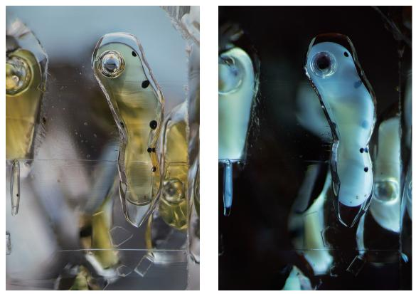
**Fig. 4** A cavity in quartz filled with petroleum. In light field (left), the petroleum displays a yellow appearance. When illuminated with the UV torch (right), in this case with the Convoy S2+, the petroleum fluoresces a chalky yellowish white, creating a totally different look and feel.
