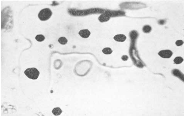
FIG. 5. Part of Fig. 4. Newly formed and parallel orientated negative crystals. 120 ×
