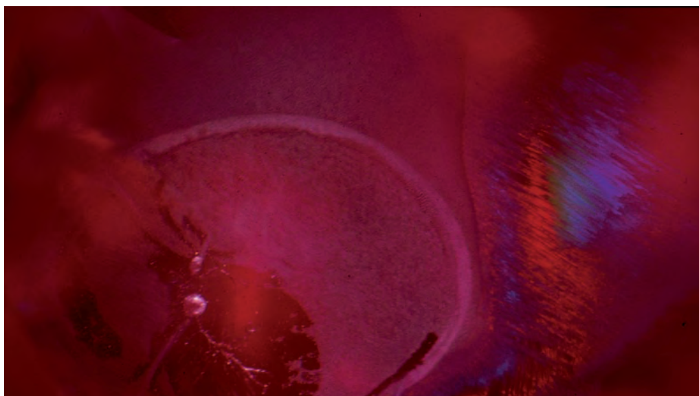
Fig. 1. This decrepitation halo surrounding a fluid inclusion in a natural, untreated Thai ruby was captured on film using a combination of darkfield and fiber-optic illumination. A Polaroid analyzer was also used to eliminate image doubling, thereby providing a sharper photo. Magnified 45X. Field of view 2.1 mm.
