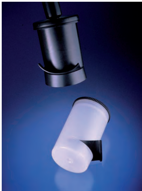
Fig. 30. Simple light shields for blocking hot spots produced by fiber-optic illuminators can be manufactured from plastic film canisters. The translucent white light shield provides diffused fiber-optic illumination, while the one constructed from an opaque black film canister provides intense direct fiber-optic lighting. Photo by Maha Tannous.
