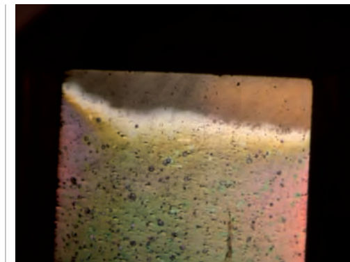
Fig. 11. Details of the gold coating on the surface of an Aqua Aura quartz are clearly visible with shadowed fiber-optic illumination. Magnified 5X. Field of view 11.2 mm.
