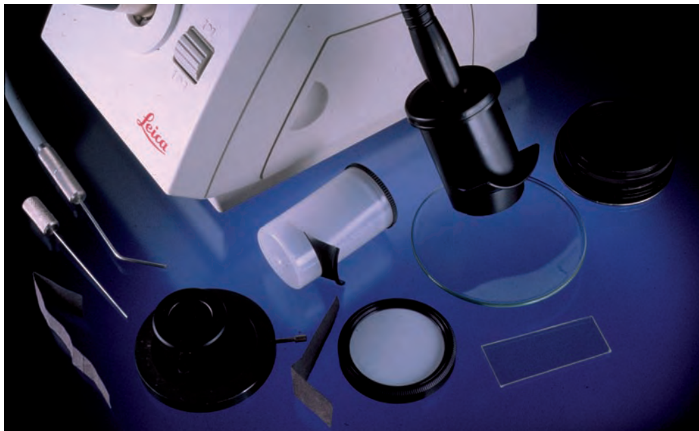
Fig. 6. This collection of lighting accessories would be found in any complete gemological photomicrographic laboratory. Shown here are a single wand fiber-optic illuminator; a pinpoint fiber-optic illuminator with two end attachments; two Polaroid plates and a first-order red compensator; a white, diffusing plate; two iris diaphragms for shadowing; two modified film cans and two black paper strips for hot spot control; and a shallow glass evaporating dish for partial immersion if needed. Photo by Maha Tannous.
