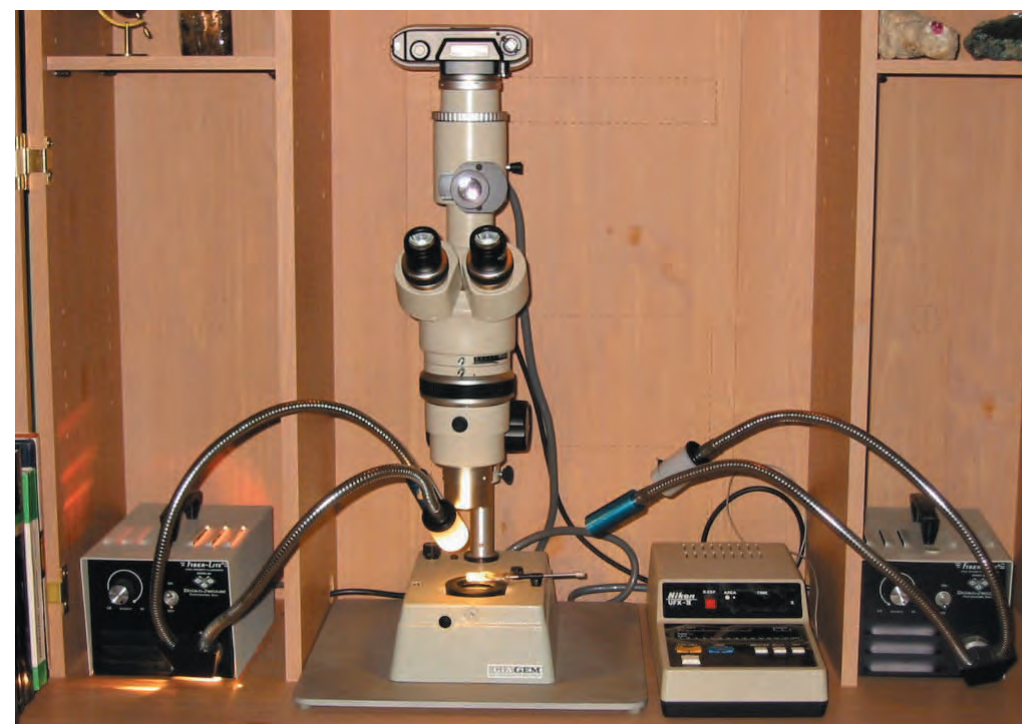
Fig. 4. Housed in a sturdy protective cabinet, the author's gemological photomicrographic system uses a trinocular arrangement so that the camera remains in place when the system is being used as a binocular microscope. Note that this custom-made darkfield and transmitted light system uses two fiber-optic illuminators (with a white film canister diffuser on the wand that is lit), but it is also easily set up for applications with polarized light, shadowing, and ultraviolet illumination. Photo by Maha Tannous.
